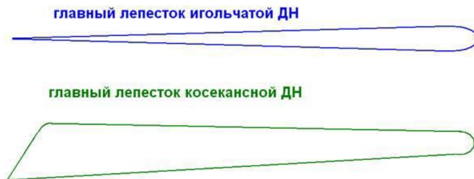
Fig. 2.2. Radiation Pattern Cross-Sections in the Elevation Plane
