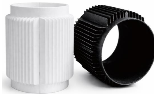
Figure 1. Polystyrene pattern and the resulting casting
